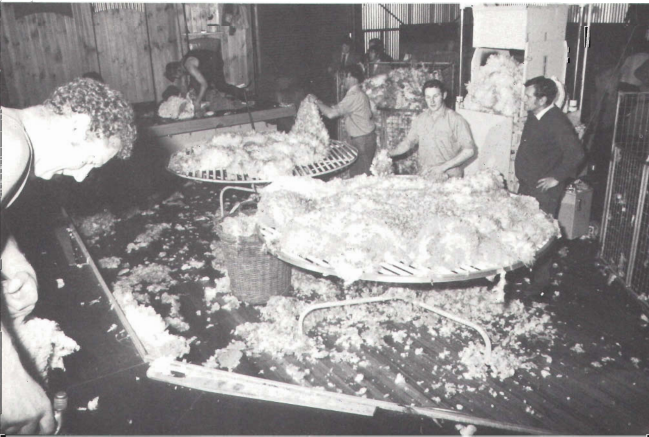
A circular shearing platform at Hillside, near Buangor, features circular swivel sorting tables, a wool press, and easy access to sheep through swing doors at the rear.
